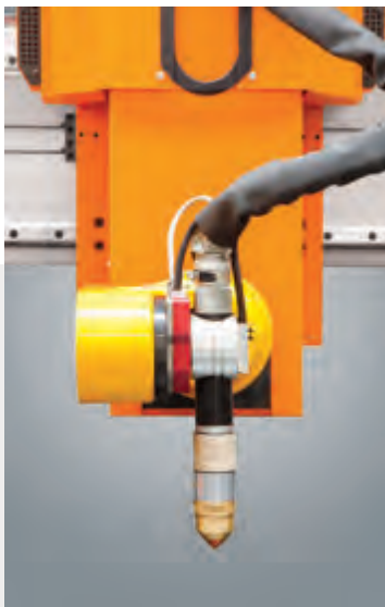
■ Cutting head moves up and down with Z axis right and left with x axis.
