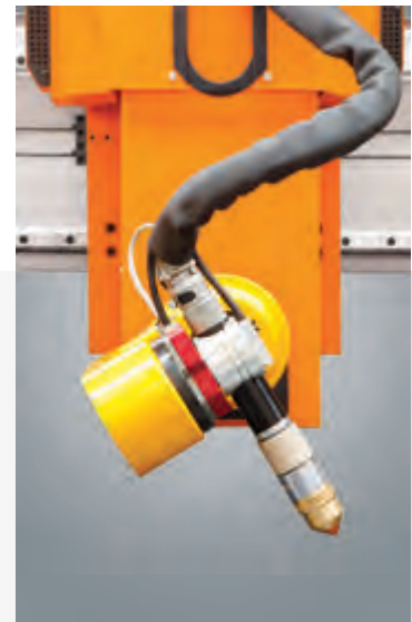
■ Can move totally \pm 50 and 60^\circ degrees at B axis.
