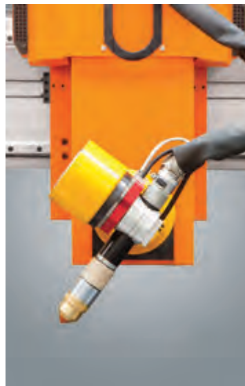
■ Can move totally \pm 50 and 60^\circ degrees at A axis.
